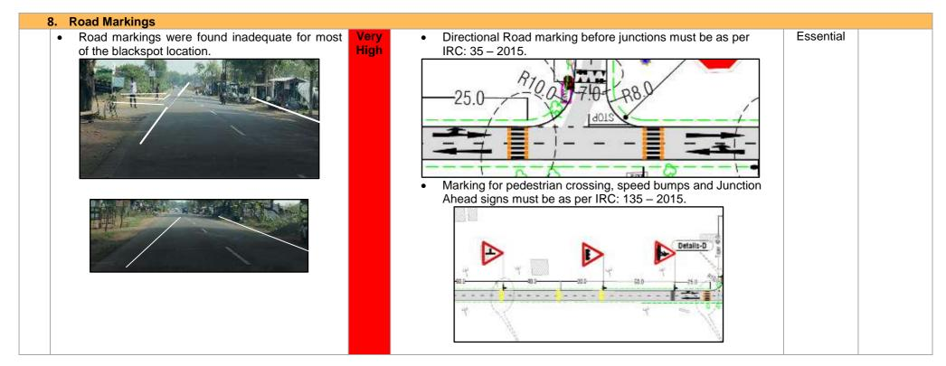
**Improvements Measures:** The above-mentioned measures will be effective for speed reduction of high-speed vehicles in built-up area and at junctions which are needed to be implement at earliest.
