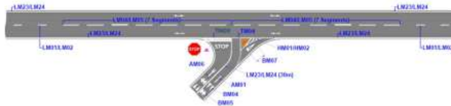
Figure 12: Typical signing and marking at Y-intersection
